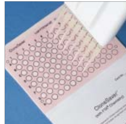
Sample Application to CloneSaver Card
